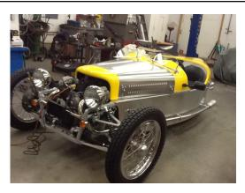
Aero Cycle Cars of England Aero Merlin Morgan three wheeler replica. Built by Steve Neal in 2014 with a Moto-Guzzi 1947cc engine with 3500 miles. Two seats side by side with disk brakes all around. Square steel tubing frame, yellow fiberglass sides with aluminum bonnet and stainless steel fenders. \$18,000 OBO. Steve Neal SKYHOOK114@comcast.net
